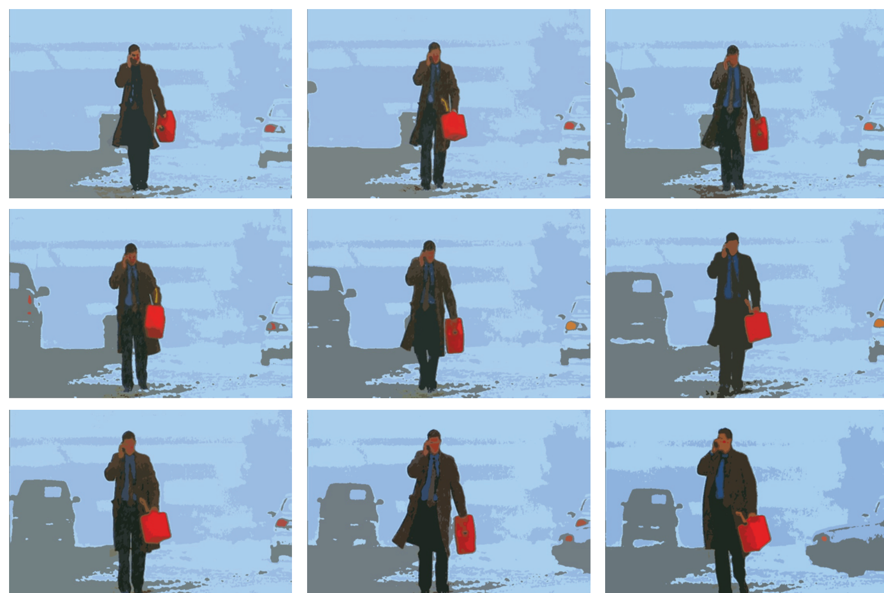
Running Recursive 2-means on an image sequence with hand-drawn saliency. Maximum recursion depth is 2 for non-salient regions and around 6 for salient regions.
