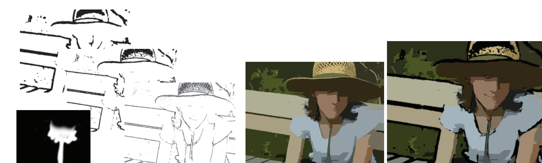
The saliency map can also be used to overlay edges computed at different scale on top of the image. A Gaussian pyramid is constructed, and edges are computed at every scale using a Sobel filter. For each pixel in the final image we select a particular scale based on saliency, with less salient regions corresponding to coarser scale.
